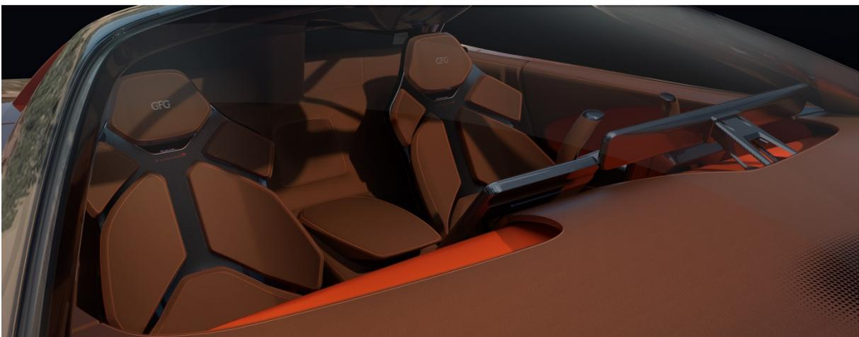
As for the interior, the two-seats-only formula offers two sporty but surprisingly comfortable seats with a special design featuring cushions fitted to a carbon structure so that driver and passenger are almost "lifted up" by the seat frame, thus ensuring comfort without sacrificing wraparound and restraining functions.
