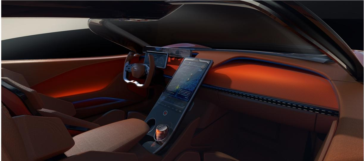
The dashboard is designed in two parts divided by an aluminum slat, which channels the air flows from the air conditioning: the upper part is a large leather wing, visually reminiscent of a horse saddle that joins up with the panels, while the lower part is made of Kult fabric in a dashing colour, in this case orange, to convey freshness, sportiness and also material innovation.
